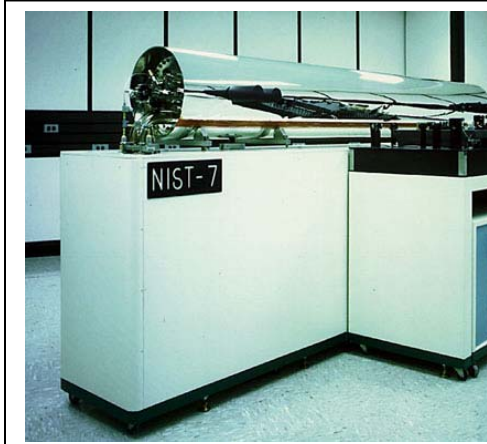
Figure 139: Atomic Clock. This atomic clock at the United States National Institute of Standards and Technology is named NIST-7. If its time were compared with a similar clock 6 million years from now, they might differ by only one second! A newer development, called NIST F-1, achieves three times greater precision by cooling the vibrating atoms to nearly absolute zero. Despite the extreme precision of atomic clocks, we have no assurance that they are not all drifting relative to “true” time. In other words, we can marvel at the precision of atomic clocks, but we cannot be certain of their accuracy.
