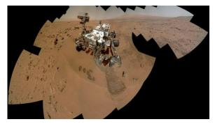
NASA's Mars rover Curiosity is a mosaic of photos taken by the rover's Mars Hand Lends Imager taken on Sol 85, the rover's 85th Martian day, as Curiosity was sampling rocks at a stop dubbed Rocknest in Gale Crater. Image released Sept. 26, 2013. (NASA/JPL-Caltech/Malin Space Science Systems)
